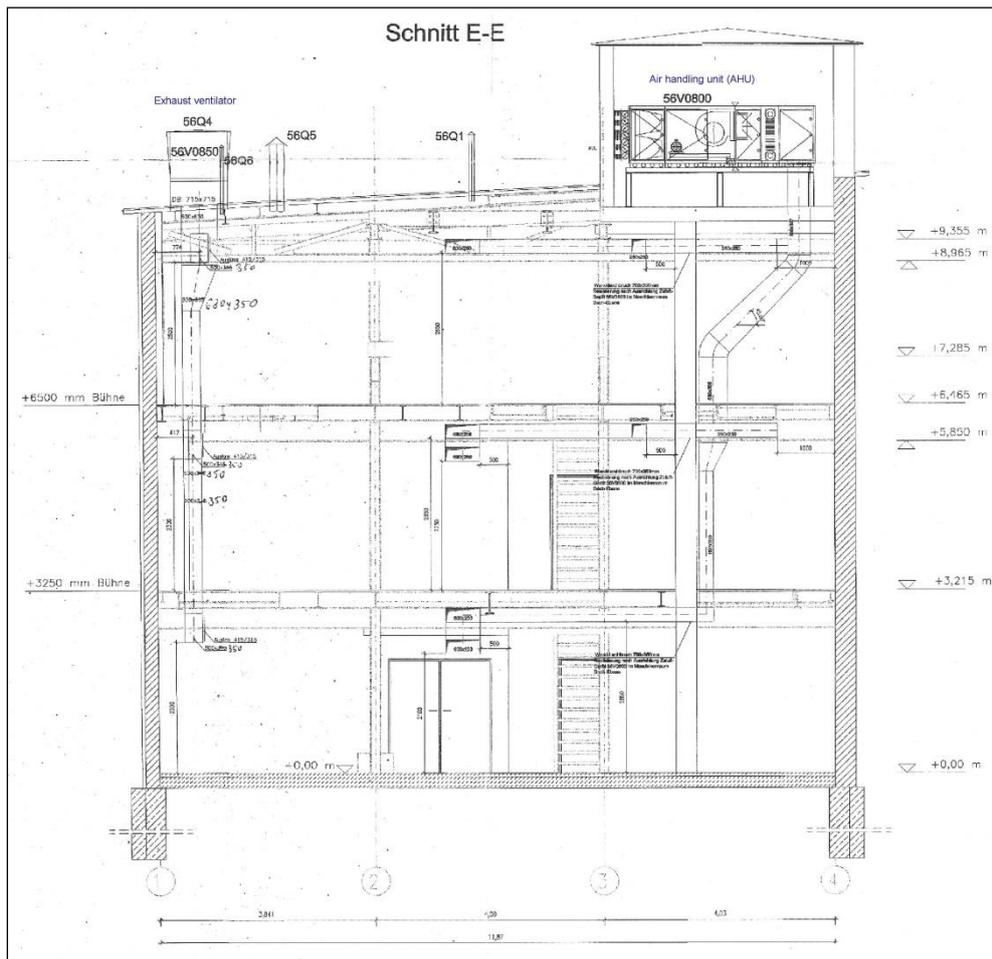
Figure 1. Cross section of the factory with air exhaust and air supply systems.
